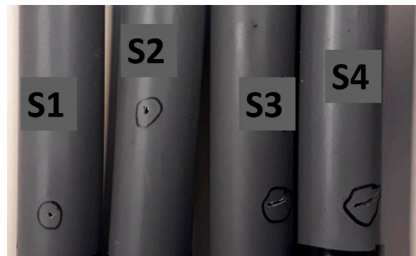
Figure 3. Samples for different leaks: S1 (1 mm), S2 (2 mm), S3 ( 4 \times 1 \text{ mm}^2 ), S4 ( 10 \times 1 \text{ mm}^2 ).
